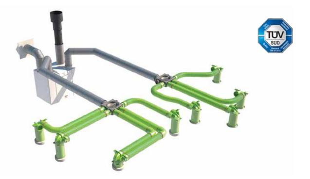
2. DB200 and DB800 universal air distribution boxes ensure maximum air distribution between the ventilation units and the connected ductwork. Restriction rings are connected directly into the distribution boxes to adjust the required flow rate per room. The air supply and air exhaust ducts, couplings and distributors are easy to connect to the distribution boxes.
